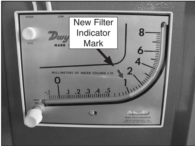
Figure 19. New filter installation mark example.
